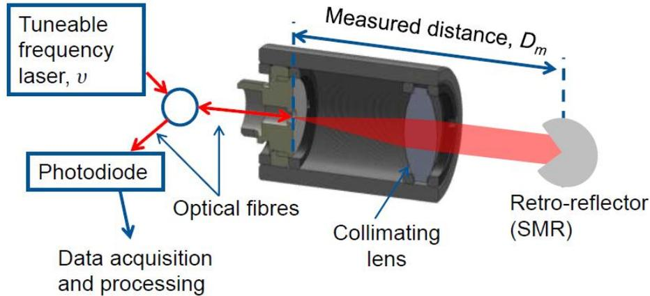
Innovative measuring system working over 10m x 10m x 5m
