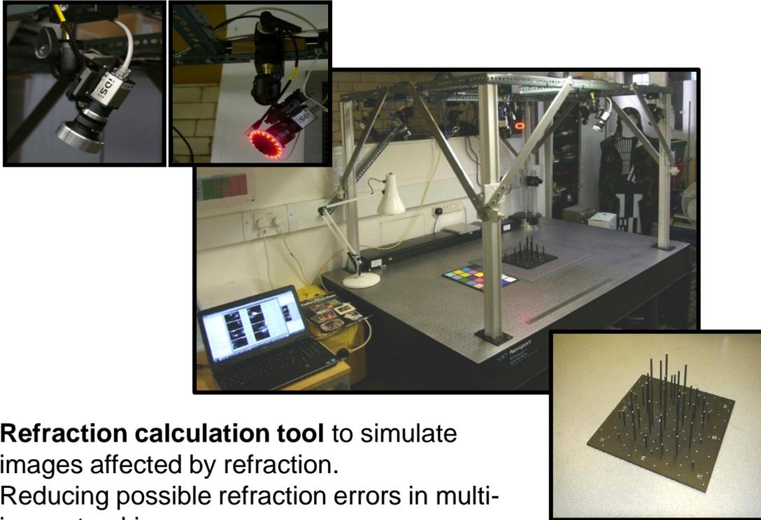
**Refraction calculation tool** to simulate images affected by refraction.
